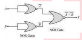
$\overline{A}$  and  $\overline{B}$  are the inputs for the last NOR gate. Hence, the output for the circuit can be written as:
